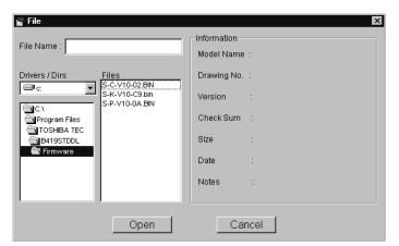
**6.** As soon as you highlight on the files in the files box, the right half of the screen will show all the data concerning the selected file as shown in the figure below.
